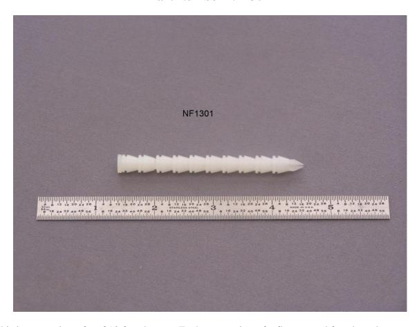
This item consists of a of 10 ferrule sets. Each set consists of a flat stepped ferrule and a graduate ferrule. **Nylon Probe Ferrules** are used to form a seal between a **Sentry Prob**e and an adapter when the Swagelok nut is tightened. It is used on all probe-to-container adapters.
